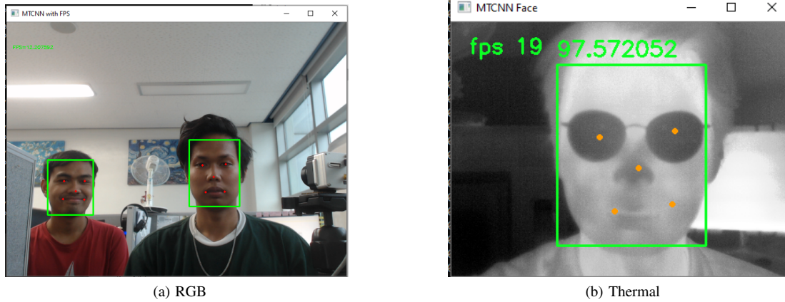
Fig. 1. Simulation of MTCNN using RGB and Thermal Camera.
